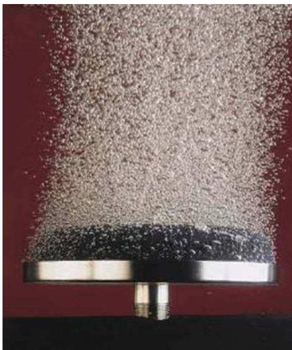
Plate 4.2 A fine bubble ozone diffuser in operation.
