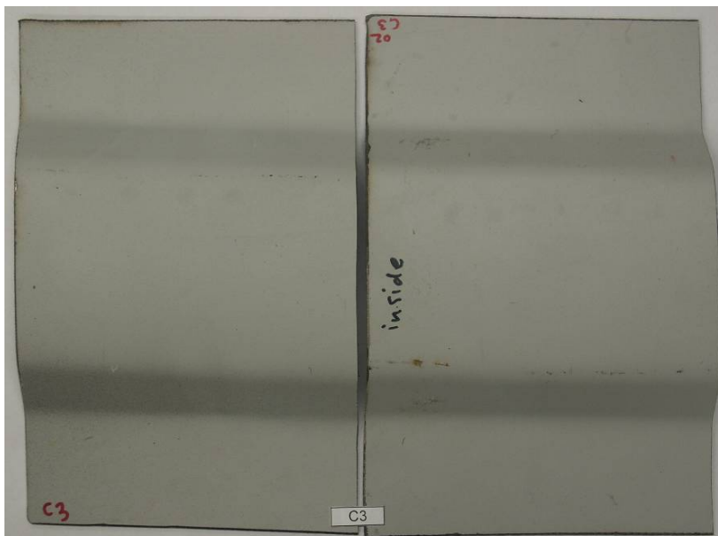
Figure A6.3. Photograph of C3. Unexposed reference specimen (left), and ozone-exposed specimen (right).
