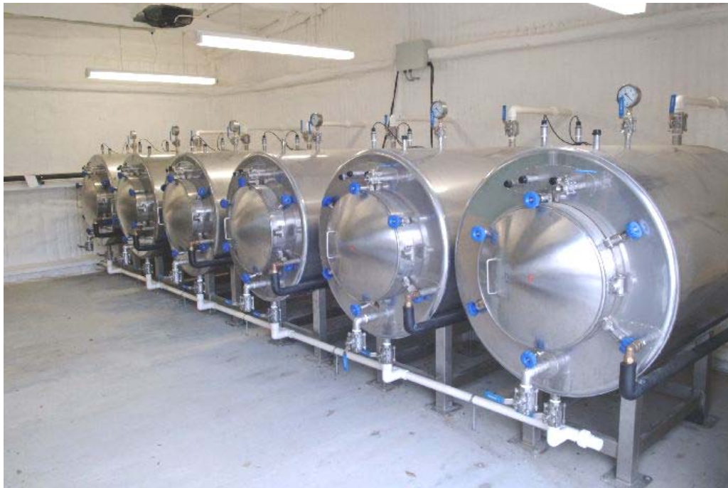
Figure 3: Chambers used for ozone experiments
