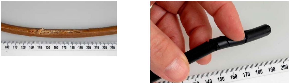
Figure 8: Chamber seals damaged by ozone treatment (left = neoprene rubber, right = nitrile rubber).
