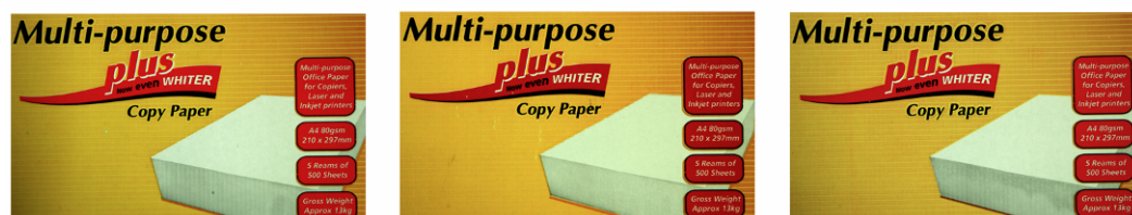
Figure 10: Bleaching of printing inks on ozone-exposed plastic-coated printed cardboard boxing relative to unexposed samples.
