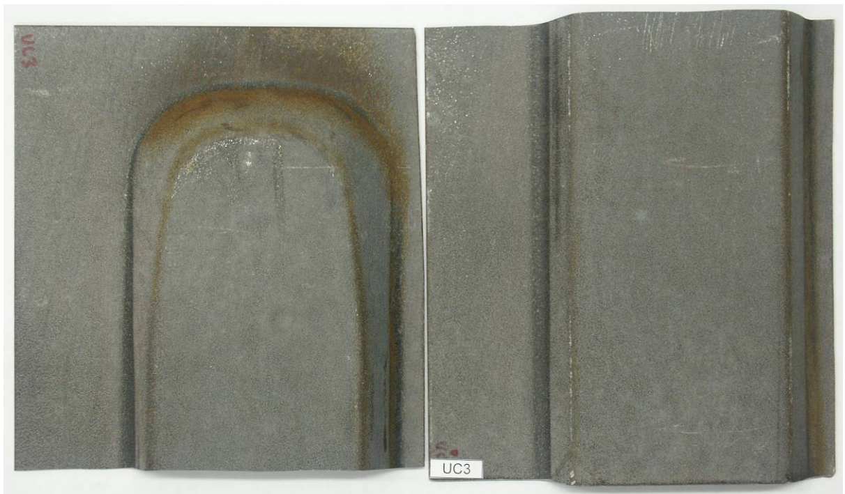
Figure A6.6: Photograph of UC3. Unexposed reference specimen (left), and ozone-exposed specimen (right).
