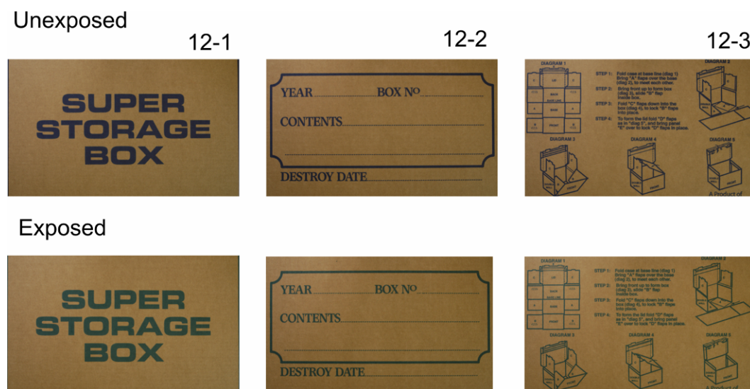
Figure 9: Bleaching of printing inks on ozone-exposed cardboard boxing.
